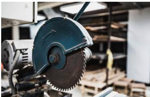
Drop saw without a self-closing guard
